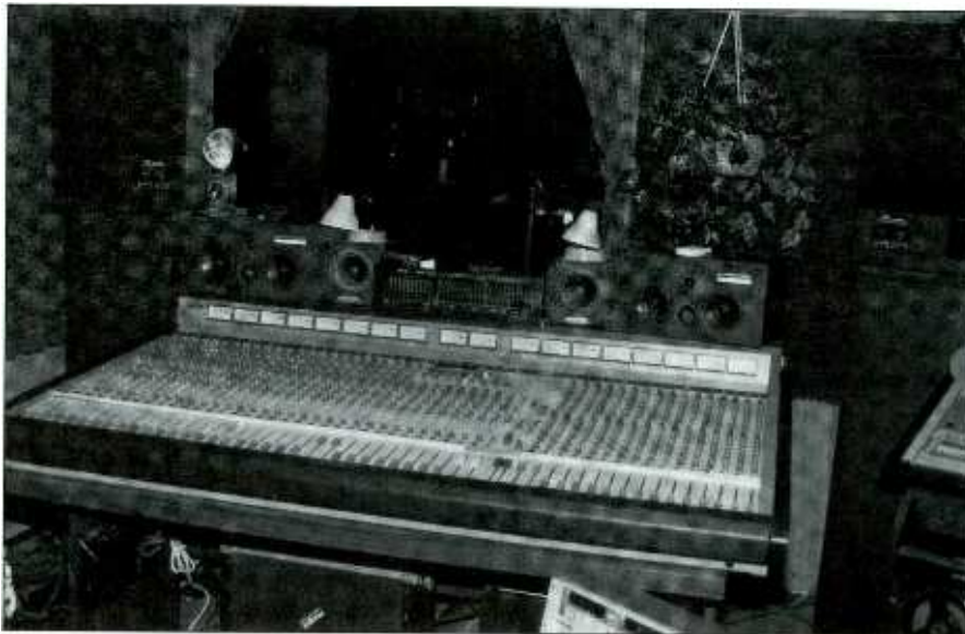
Figure 1. The Sunset Ridge control room. Tascam M600 console and GA30 EQ with Auratone and Westlake Audio speakers.
