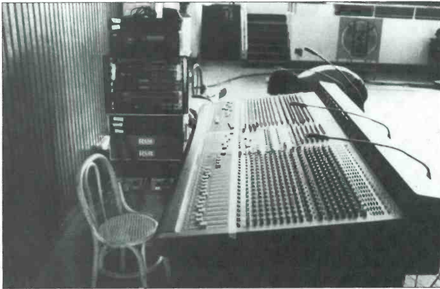
Figure 4. A Yamaha PM-3000 40-channel console, along with Rane crossovers and graphic equalizers, equipped the house mix point at the Show TEKNIX mix point.
