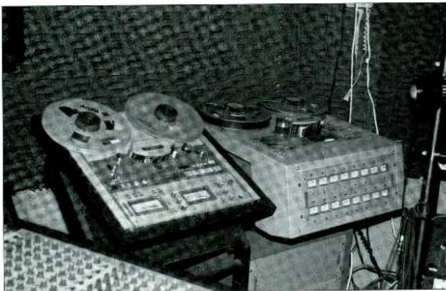
Figure 2. A Tascam 42B 2-track and MS-16 16-track are to the right of the console.
